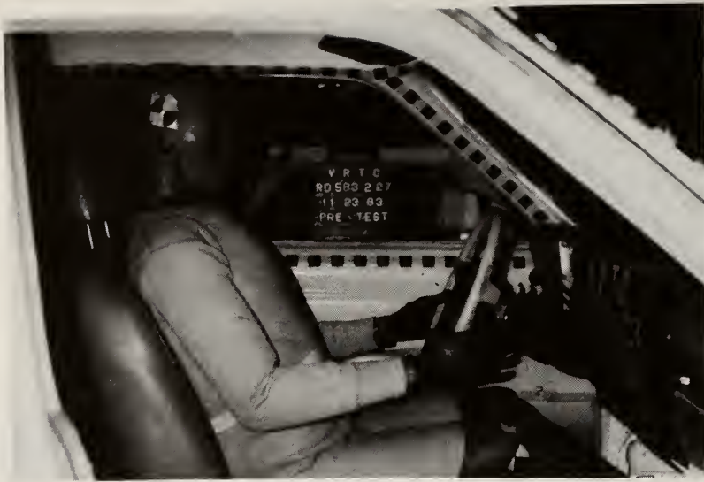
Dummy Positioning Pre Test 27
